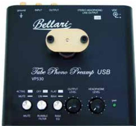
All the same features as the VP130, but with the addition of a RIAA EQ switch to have the availability to use RIAA or a flat un EQ'd signal with the VP530. USB output to plug directly into your computer.
