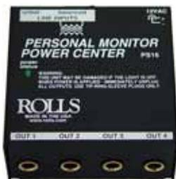
The PS16 will power and supply signal to up to four of the PM50s, PM55, or PM351 units directly, and with the optional "Y" adapter up to eight. The power is provided on the ring of the jack. The PM series units must operate in mono.
