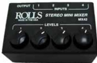
The MX42 is a passive stereo resistance mixer that will attenuate the volume of each channel to one output. Ideal for mixing hot line level signals. It will also work in reverse, passively distributing a single stereo signal to four stereo outputs.
