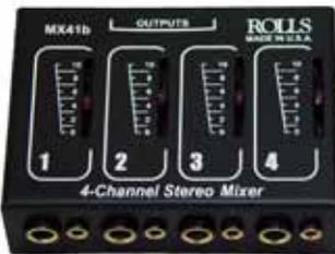
The MX41b is a passive stereo resistance mixer that will attenuate the volume of each channel to one output. Ideal for mixing hot line level signals. It will also work in reverse, passively distributing a single stereo signal to four stereo outputs.
