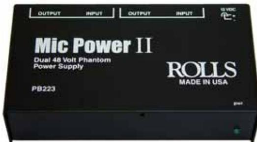
The PB223 has the same design as the PB23 just with 2 channels. As with most of the Rolls products, the power supply is included with the unit.
