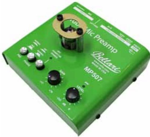
The MP507 is a single channel preamp that utilizes a single 12ax7 vacuum tube. It has a MU-Metal audio transformer to decrease noise and enhance the sound quality of the XLR input. The design of the MP507 utilizes a high speed self regulated switching power supply to generate 230V of clean usable plate voltage for the 12ax7 vacuum tube. The result is a clean and powerful sounding tube preamp.
